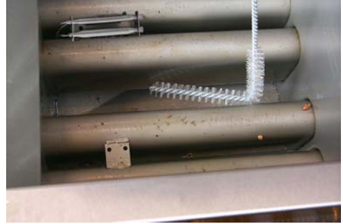
Use the L-shaped brush to loosen debris as oil drains from the frypot.
